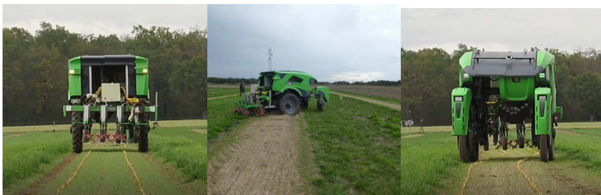
Picture 3: Field navigation experimentation with SITIA Trektor (a pass in straight line, a half turn controlled manually and a pass on curve line after half turn)
