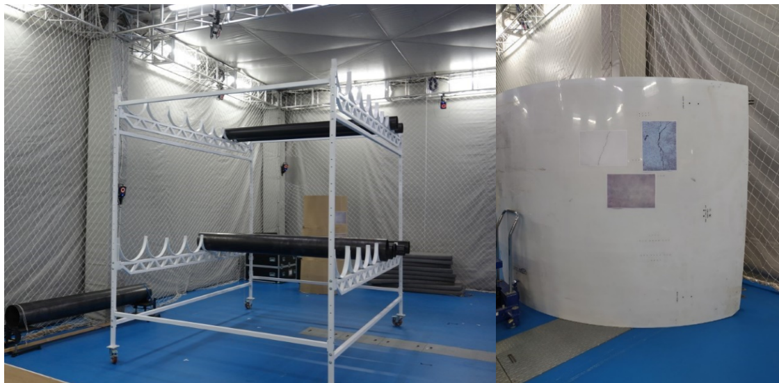
Figure 6. Pipe rack used as obstacle (left). Structure used as point of interest with defects (right).
