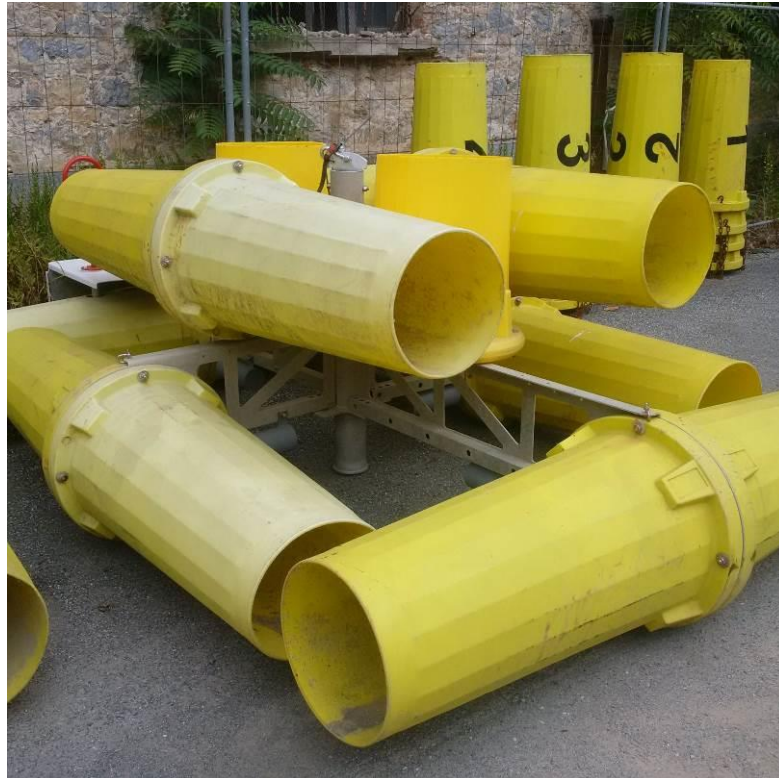
Figure 5. Piping assembly structure. The structure, composed of yellow pipes, has the following dimensions: 2 m (front area) x 3 m x 1.8 m (height).
