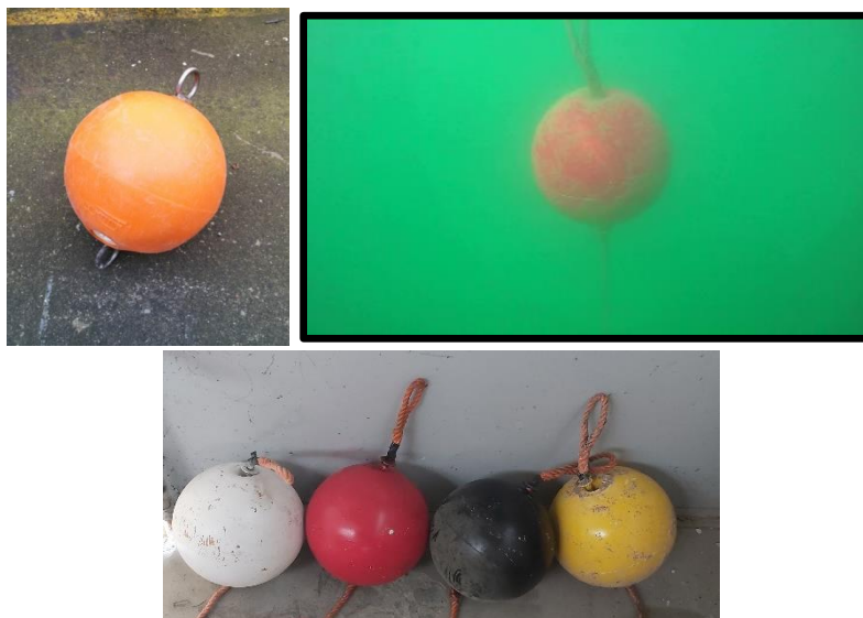
Figure 4. Image of the buoy outside of the water (top-left) used for the gate and of a red buoy underwater (coloured buoys in the “buoy area”)(top-right). The OD of the sphere is about 30 cm. (Bottom) the buoys with four possible colours.
